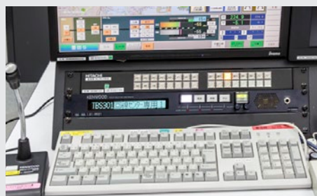
The TCN-371 that is set with a mic shows at-a-glance display of the other party's terminal and user name.
