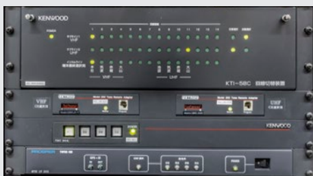
Rack featuring a Prosper interface box and base station line-switching device
